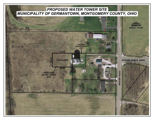
Figure 3. Project location – Existing water tower and 0.344-acre site marked for proposed tank
